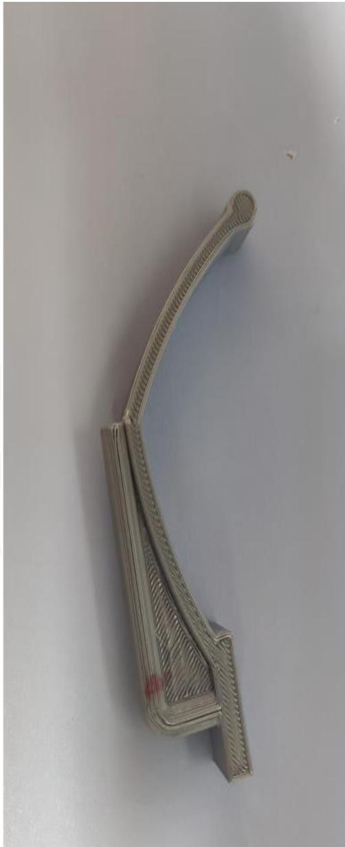
Figure 4.26 Samples after three point bending
