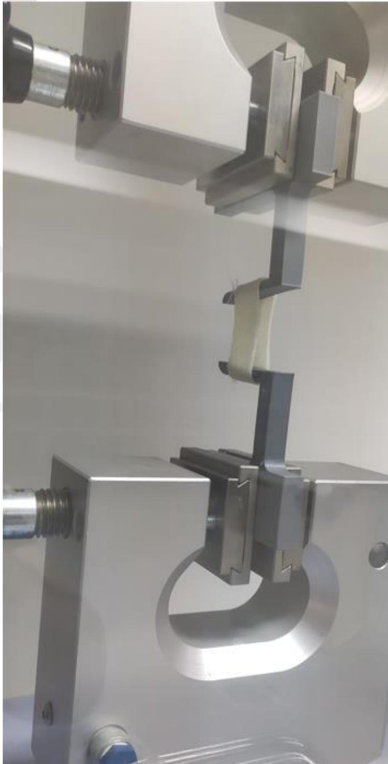
Figure 3.31 Tensile behavior test of aorta parts with holder
