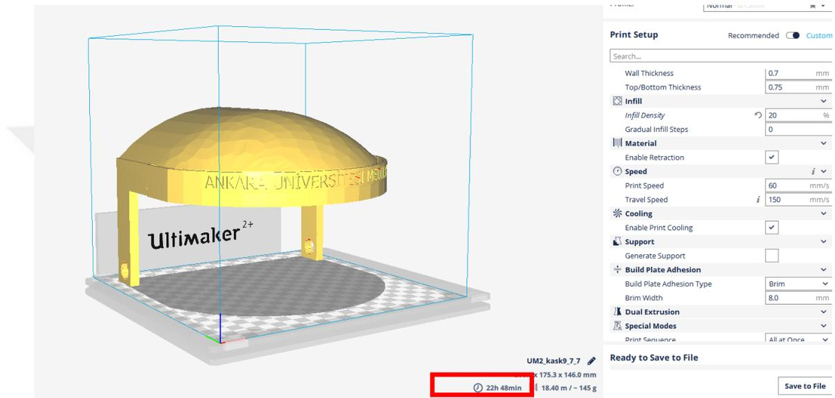
Figure 4.2 3D printing procedure time of head covered main body
