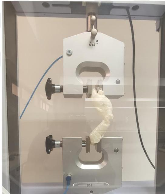
Figure 3.29 Tensile behavior test of aorta parts
