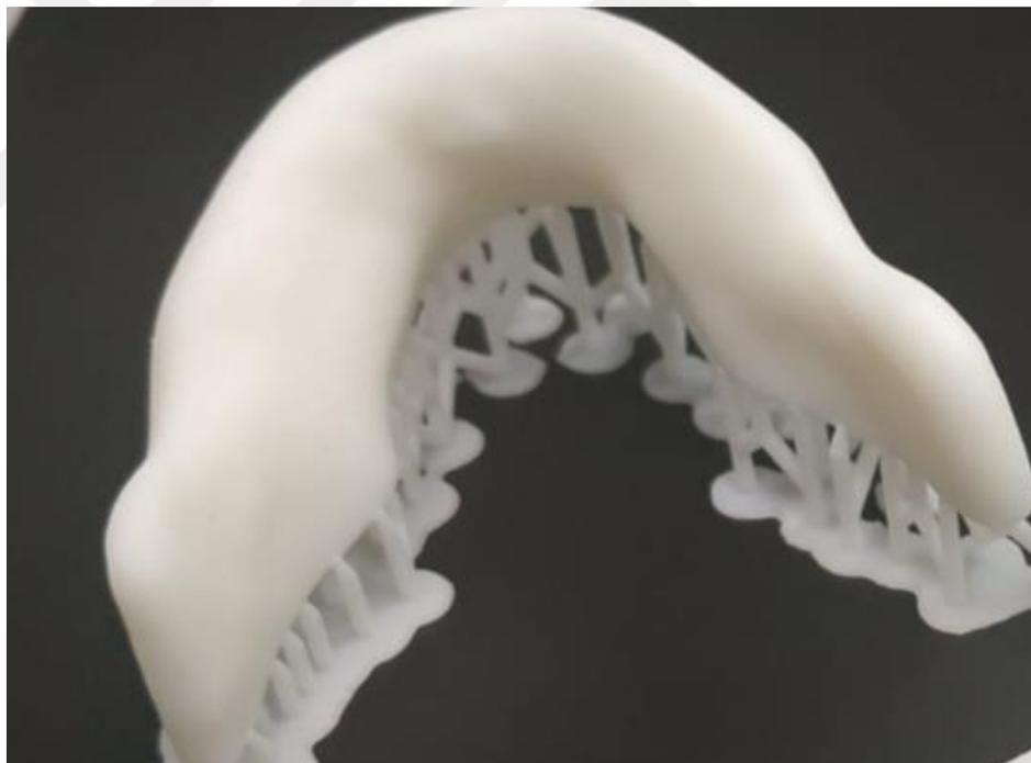
Figure 2.3 3D printing of human mandibula with SLA in our laboratory
