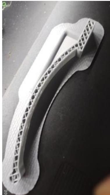
Figure 3.34 3D printing with 25% infill rate
